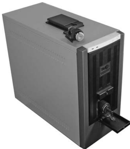
FIG.1: Automated ballistic identification system “TAIS”.
